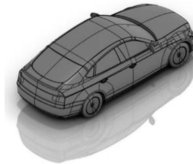
Figure 2: CAD Isometric model of DrivAer Fastback Car
